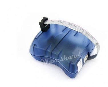
AVR ISP Programmer, compatible with AT AVRISP from ATMEL, supports AVR Studio 4/5/6/7
