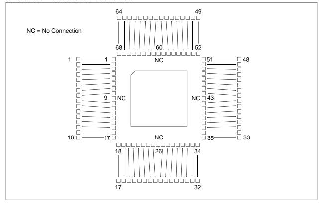
FIGURE 31: HEADER TO 80-PIN TQFP
