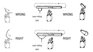
Cam or dog arrangements should be such that the actuator is not suddently released to snap back freely.
