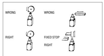
For limit switches with pushrod actuators, the actuating force should be applied as nearly as possible in line with the pushrod axis.
