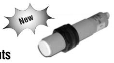
The new 944 series are microprocessor controlled and fully programmable by teach-in, with the simple pressing of a button. They offer analogue and two switching outputs through a standard M-12, 5-pin connector. All the models are IP67 with chemical-resistant body and epoxy face. Parameters are stored in non-volatile memory.
