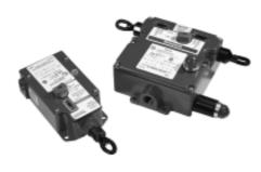
CPS Series Cable Pull Safety Switches provide a readily accessible emergency stop signal. This is a costeffective means compared to using multiple emergency stop push-buttons. (Cable Pull Safety Switches are not, however, to be used as a means of personnel safeguarding. They may be used to prevent further injury or damage to equipment when used for emergency stop signaling.)
