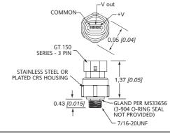
**MEASUREMENT TYPE** PRESSURE RANGE 0 psig to 5,000 psig REFERENCE BE-4R5000PG6DS Gauge
