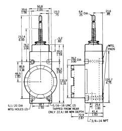
Operating force max. (OF): Pretravel max. (PT): Operating temperature: 2,78 N (10 oz) 25,4 mm (1.0 in) -12 °C to 93 °C (10 °F to 200 °F)
