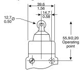
Pretravel: 1,78 mm (0.07 in) max. Differential travel: 0,38 mm (0.015 in) max. Overtravel: 4,83 mm (019 in) min. **Operating point:** 55,9 mm ± 1,02  $2.20 \text{ in } \pm 0.04$
