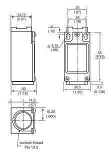
Mechanical life: up to 10 million Sealing: IP 66, NEMA 1, 4, 12, 13 Operating temperature: -25 °C to 85 °C -13 °F to 185 °F
