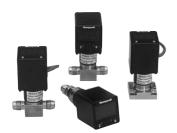
With space at a premium in semiconductor gas distribution systems, the Series TLD pressure transducer with local display offers an integrated solution that reduces the overall height of the transducer/display assembly to as little as 3.5 in [88,9 mm]. To accomplish this, the transducer's signal amplifier is mounted within the display, with the added benefit of zero and span adjustments conveniently located on the LED display face.
