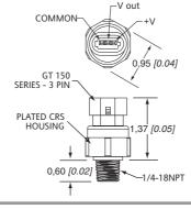
**MEASUREMENT TYPE** PRESSURE RANGE REFERENCE BE-4R125PG5DC Gauge 0 psig to 125 psig
