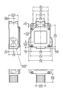
Mechanical life: up to 1 million IP 66, NEMA/UL 1, 4, 12, 13 Sealing: Operating temperature: -25 °C to 85 °C
