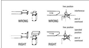
Operating mechanisms for limit switches shoud be so designed that, under any operating or emergency conditions, the limit switch is not operated beyond its overtravel limit position. A limit switch should not be used as a mechanical stop.
