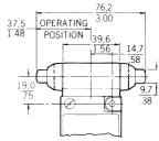
LSG contact transfer is maintained after either plunger is operated. Operation of other plunger resets switch.
