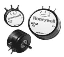
Available in servo mount styles, the WPM Series rotary transducer provides long life by utilizing the proprietary MystR® conductive plastic film, precious metal wipers and shielded ball bearings on the stainless steel shaft.
