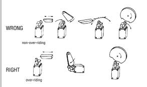
For limit switches with lever actuators, the actuating force should be applied as nearly perpendicular to the lever as practical and perpendicular to the shaft axis about which the lever rotates.
