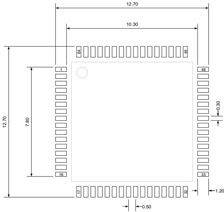
(Original dimensions are in millimeters)
