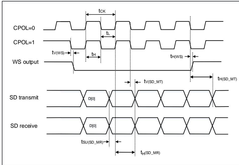
Figure 4-11. I2S timing diagram - slave mode
