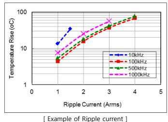
2) The rise in increase by self-heating of MLCC must not exceed  $20^{\circ}$ C
