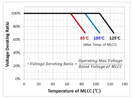
[Example of derating graph for derated MLCC] \* Vmax ≤ Derated Voltage
