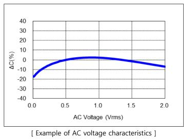
\* Sample : X5R 10uF, Rated voltage 6.3V
