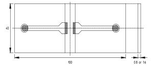
(Substrate for bending strength test)
