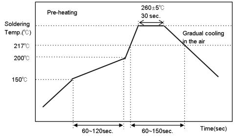
[Reflow Soldering Conditions]
