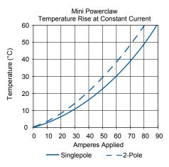
NOTE: Temperature rise charts are based on a 25°C ambient temperature. Powerclaw charts are based on #8 AWG equivalent copper foil on board side, mated to #6 AWG conductor on wire side.
