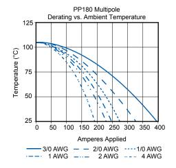
NOTE: Temperature rise charts are based on a 25°C ambient temperature.
