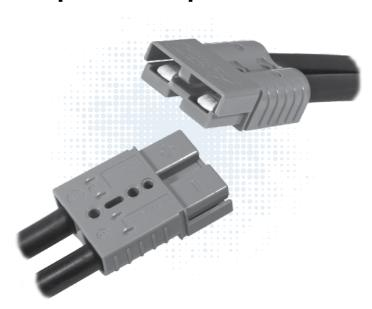
Like the other Multipole connectors, the SB®120 offers color-coded mechanically keyed housings. Keys can be used to identify and separate different circuits, or prevent users from accidentally cross mating different voltages. Wires sizes from #10 (5.3 mm²) to #1 (42.4 mm²) are held in the second smallest SB® housing.
