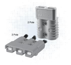
Wires sizes from #10 (5.3 mm²) to 1/0 (53.5 mm²) fit in the second to largest connector in the SB® series. The 3 pole SB®175 adds an additional position for power or grounding. All Multipole wire connector housings are genderless and mate to themselves minimizing inventory and assembly complexity.
