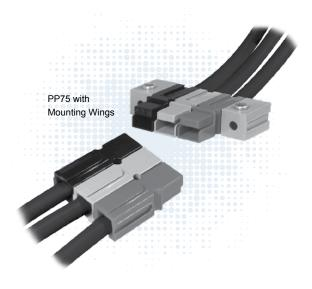
PP75 series Powerpole® housings can be used for wire-to-wire, wire-to-board, and wire-to-busbar applications. Wire sizes from #16 AWG (1.3 mm²) to #6 (13.3 mm²) offer power capabilities up to 120 amps per pole. Locking housings offer the capability to secure Powerpole® housings to each other and to mounting pads. Housings made from chemical resistant (CR) resin withstand industrial solvents better than standard housings.
