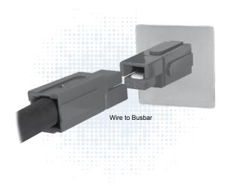
PP180 are the largest of the Powerpole® series housings. They are designed to accommodate up to 3/0 (70 mm²) wires and handle high currents up to 350 amps. Busbar contacts are also available for power inputs and takeoffs. Color-coded housings minimize user confusion and the potential of cross mating circuits.
