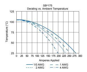
NOTE: Temperature rise charts are based on a 25°C ambient temperature.
