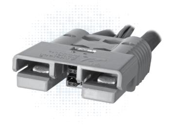
SBX® and SBE® connectors can integrate up to 8 auxiliary power / signal contacts along with the two primary power circuits. SBE® connectors feature an IEC 60950 touch safe housing molded from a chemical resistant PBT/PC blend resin. SBX® are molded from a rugged PC resin and are rated IP20 per IEC 60529.
