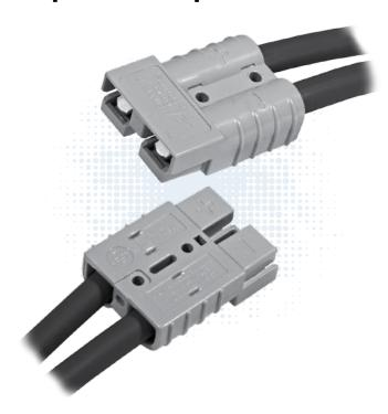
Based off the design pioneered by Anderson in 1953, APP®'s two pole SB® connectors set the standard for DC power distribution and battery connections. SB®50 connectors feature a one piece plastic housing using stainless steel springs to hold low resistance contacts in place. Wires sizes from #16 (1.3 mm²) to #6 (13.3 mm²) are held in the smallest of the SB® series housings.
