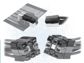
PP15-45 series are the smallest Powerpole® housings. They can be used for wire-to-wire or wire-to-board applications. Wire sizes from #20 AWG (0.75 mm²) to #10 (6 mm²) offer power capabilities up to 55 amps per pole. Finger proof housings and the ability to incorporate first-mate last-break ground connectors enhance the capabilities of this Powerpole® series.
