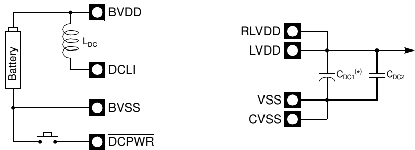
Figure 8. Battery DC-DC Connection
