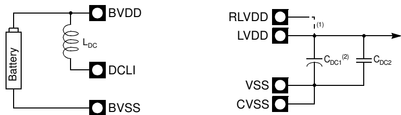
Figure 135. Battery DC-DC Connection
