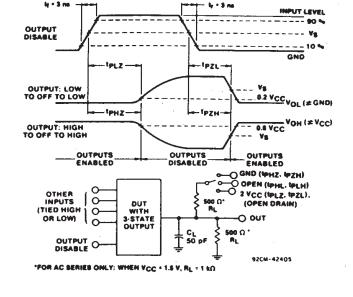
Fig. 1 - Simultaneous switching transient waveforms.
