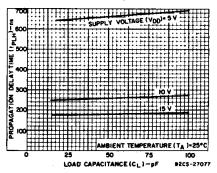
Fig. 2 — Typical data-to-output, low-to-high-level propagation dalay time as a function of load capacitance.
