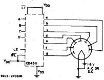
A medium-brightness intensity display can be obtained with low-voltage fluorescent displays such as the Tung-Sol Digivac S/G\*\* Series.
