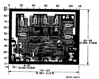
Dimensions and pad layout for CD45118 chip.
