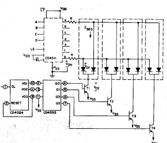
Multiplexing Scheme Showing 2 of 7 Segments Connected
