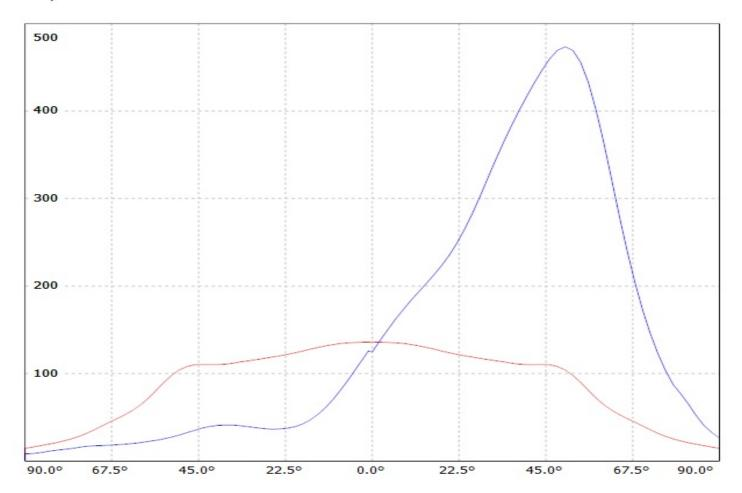
Luminaire: Ledil Oy CA12087-Strada-FW-Tape-XP Lamps: 1 x Cree XP-E 74,6lm 250mA
