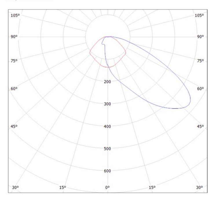
Luminaire: Ledil Oy CA12087-Strada-FW-Tape-XP Lamps: 1 x Cree XP-E 74,6lm 250mA
