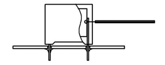
Temperature monitored inside the capacitor.
