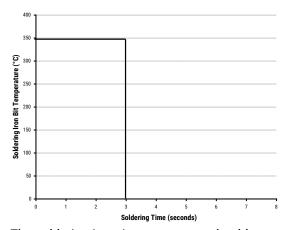
The soldering iron tip temperature should be set at 350°C (+10°C) maximum with the soldering duration not to exceed more than 3 seconds.
