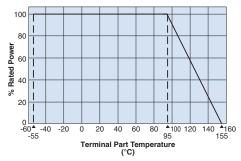
When the terminal part temperature of the resistor exceeds the rated terminal part temperature shown above, the power shall be derated according to the derating curve. Please refer to "Introduction of the derating curve based on the terminal part temperature" in the beginning of our catalog before use.
