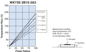
Regarding the temperature rise, the value of the temperature varies per conditions and board for use since the temperature is measured under our measuring conditions.
