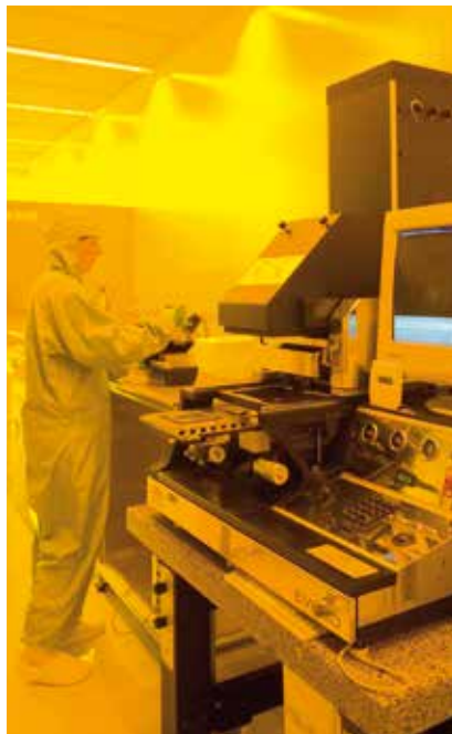
Photolithography: creating the structure on the substrate
