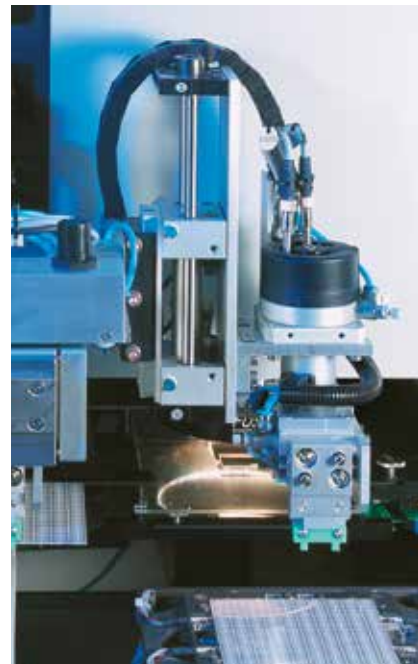
Laser trimming of platinum-chip temperature sensors
