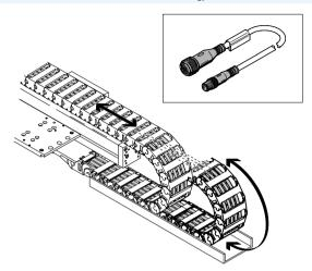
Energy chain applications involve high mechanical loads, particularly if the energy chains have small radii. It is possible that the connecting cable may be used in an environment where it is subject to continuous bending.
