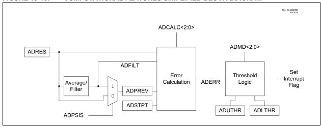
The operation of the ADC computational features is controlled by MD <2:0> bits in the ADCON2 register.
