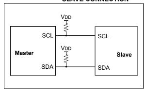
On the last byte of data communicated, the master device may end the transmission by sending a Stop bit. If the master device is in Receive mode, it sends the Stop condition in place of the last  $\overline{ACK}$  bit. A Stop condition is indicated by a low-to-high transition of the SDA line while the SCL line is held high.
