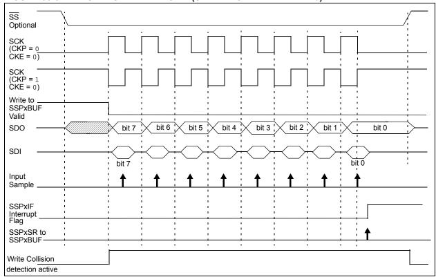
FIGURE 33-10: SPI MODE WAVEFORM (SLAVE MODE WITH CKE = 1)
