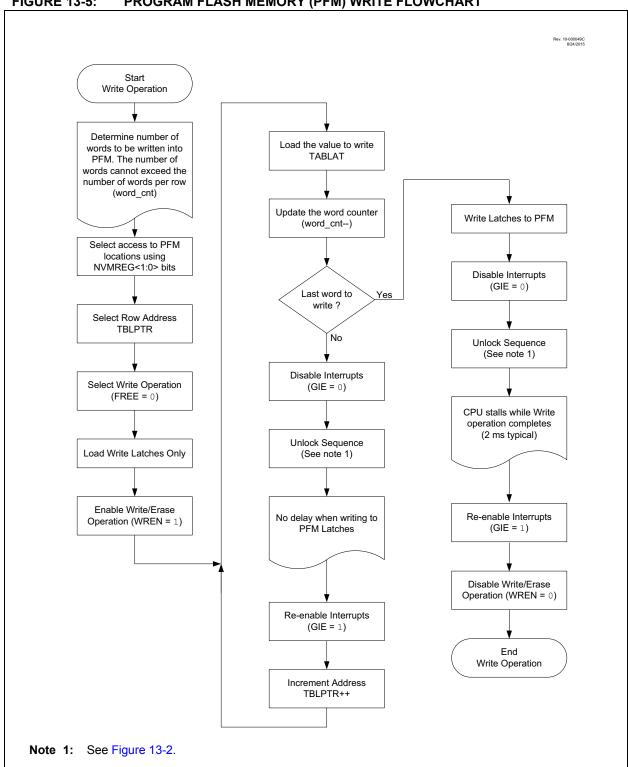
**FIGURE 13-5:** PROGRAM FLASH MEMORY (PFM) WRITE FLOWCHART
