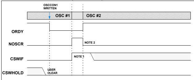
Note 1: CSWIF is asserted coincident with NOSCR; interrupt is serviced at OSC#2 speed.
