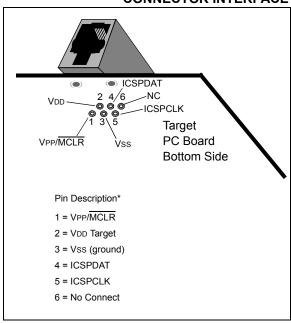
Another connector often found in use with the PICkit™ programmers is a standard 6-pin header with 0.1 inch spacing. Refer to Figure 36-2.
