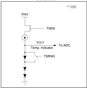
The output of the circuit is measured using the internal Analog-to-Digital Converter. A channel is reserved for the temperature circuit output. Refer to Section 19.0 "Analog-to-Digital Converter with Computation (ADC2) Module" for detailed information.
