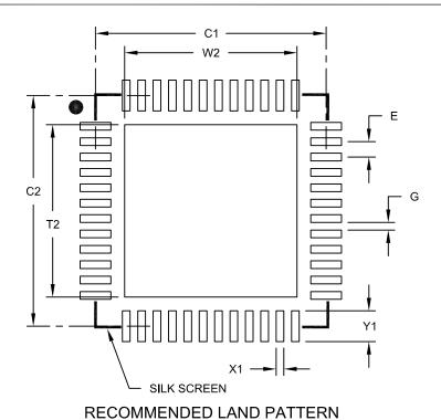
MILLIMETERS Units MIN **Dimension Limits** MOM MAX 0.40 BSC Contact Pitch Ε Optional Center Pad Width W2 4.45 Optional Center Pad Length T2 4.45 Contact Pad Spacing C1 6.00 Contact Pad Spacing C2 6.00 Contact Pad Width (X28) X1 0.20 Contact Pad Length (X28) Y1 0.80 Distance Between Pads G 0.20
