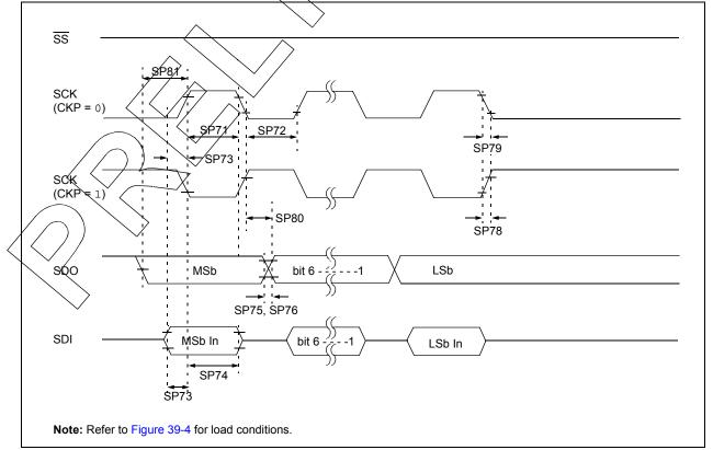
FIGURE 39-19: SPI SLAVE MODE TIMING (CKE = 0) SS SP70 SCK SP83 (CKP = 0)SP72 SP78 SP79 SCK (CKP = 1) SP78 SP79 SP80-SDO MSb bit 6 SP75, SP76 SP77 SDI MSb In bit 6 LSb In SP74 SP73 Note: Refer to Figure 39-4 for load conditions.
