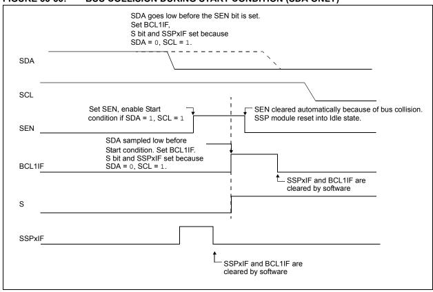
FIGURE 33-34: BUS COLLISION DURING START CONDITION (SCL = 0)
