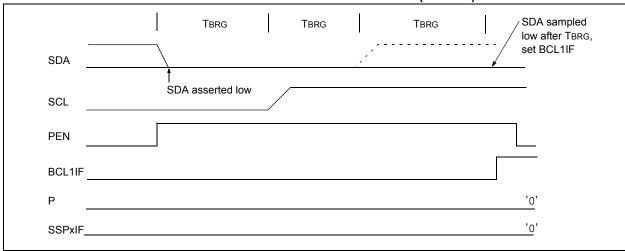
FIGURE 33-39: BUS COLLISION DURING A STOP CONDITION (CASE 2)
