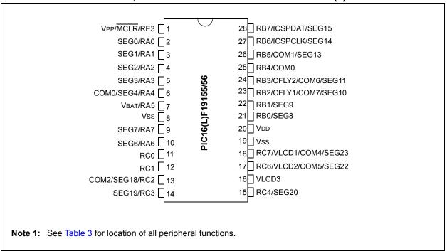
FIGURE 2: 28-PIN UQFN PIN DIAGRAM FOR PIC16(L)F19155/56
