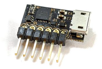
It features the Silicon Labs CP2102N chip for excellent cross platform driver support, on-board autoprogram circuitry to transparently handle device programming and serial console use, a V+ blocking diode and ESD protection.
