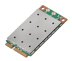
EWM-W158F01E is an Industrial-Grade 802.11a/b/g/n 2.4GHz + 5GHz Mini Card based on Qualcomm Atheros AR9592-AR1B chipset. It supports 2T2R (2x2) MIMO spatial multiplexing technology, which runs up to 300Mbps and delivers superior WiFi output power up to 19dBm.
