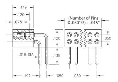
**Description:** Interconnect Socket Right Angle Socket Accepts .015"- .020" (0,38 - 0,508 mm) dia leads Double Row Through Hole
