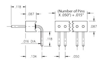
**Description:** Interconnect Header Right Angle Pin Header .016" (0,41mm) Pin Head Single Row Through Hole Plating Code: 10 Shell Plating: 10  $\mu$ " Gold over 100  $\mu$ " Nickel
