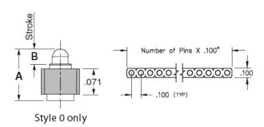
**Description:** Interconnect SLC Header Spring-Loaded Header Vertical Mount SMT Single Row Surface Mount **Plating Code:** Shell Plating:  $20\mu$ " Gold over  $100\mu$ " Nickel Inner Spring Plating: 10µ" Gold
