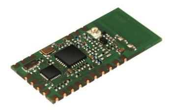
XTR-8LR-ENC is a transceiver based on  $LoRa^{TM}$  modulation able to guarantee very long range communication (8 Km line of sight), high interference immunity, very high sensitivity and very low current consumption.
