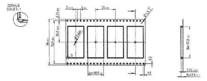
Figure 4: tape and reel drawing (in mm)
