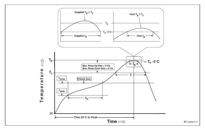
Figure 3: Soldering profile for XTR-8LR-ENC
