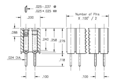
**Description:** Interconnect Socket Standard Solder Tail Socket Accepts .025" - .037" (0,635 - 0,94 mm)dia leads Double Row Through Hole
