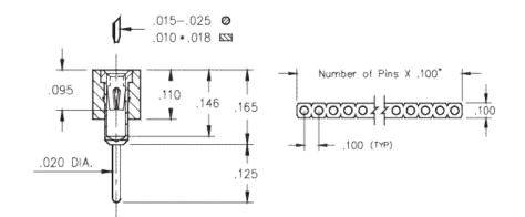
**Description:** Interconnect Socket Standard Solder Tail Socket Accepts .015"- .025" (0,38 - 0,635 mm) dia leads Single Row Through Hole Plating Code: Shell Plating: 10  $\mu$ " Gold over 100  $\mu$ " Nickel Inner Contact Plating:
