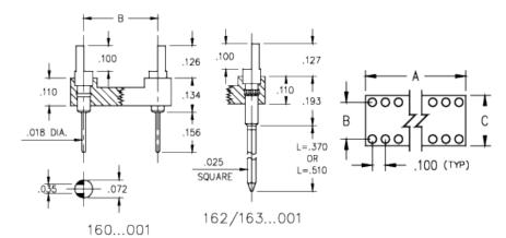
**Description:** DIP Dual In Line Header Solder Tail DIP Header Slotted Head Open Frame Through Hole Plating Code: 10
