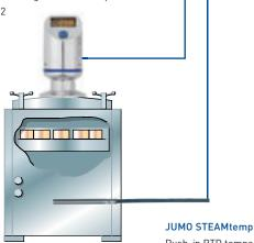
Push-in RTD temperature probe in steam-tight version Type 902830
