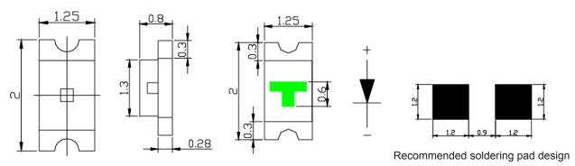
Dimensions : Millimetres Tolerance: ±0.2mm
