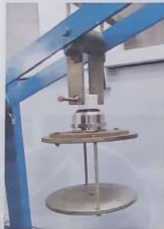
Typical Set-up for Cable Retention Test
