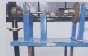
Typical Set-up for Cable Anchorage Twist Test
