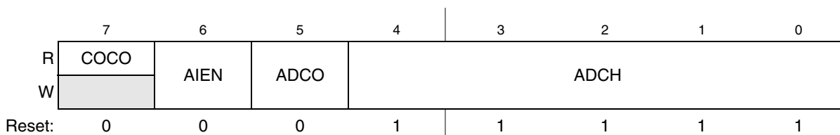
Figure 10-3. Status and Control Register (ADCSC1)
