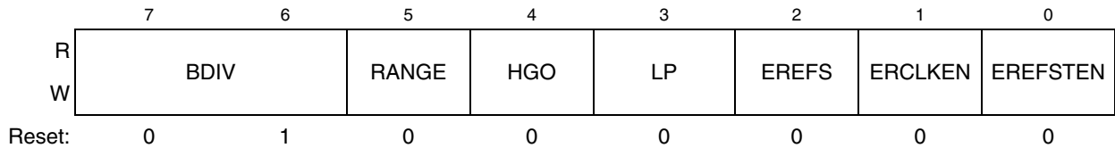
Figure 12-4. MCG Control Register 2 (MCGC2)
