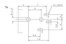
printed circuit board layout, components side view
