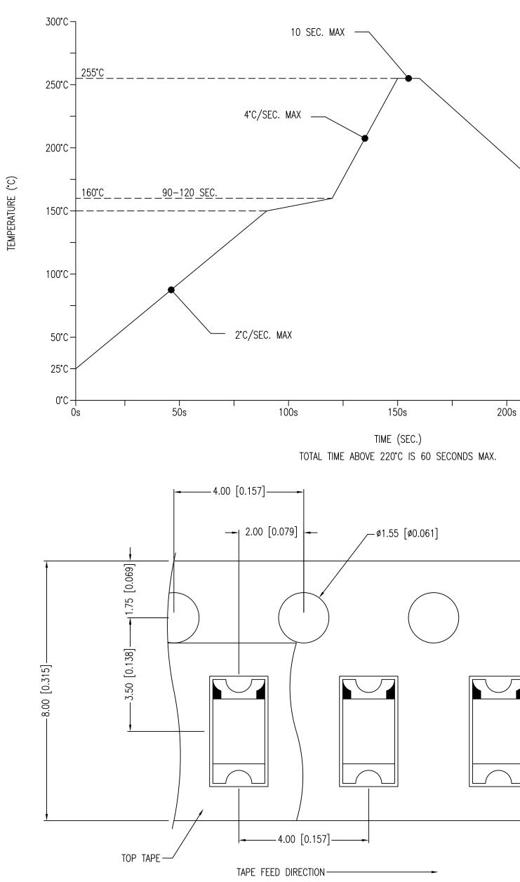
\*UNLESS OTHERWISE SPECIFIED TOLERANCES PER DECIMAL PRECISION ARE: X=±1 (±0.039), X.X=±0.5 (±0.020), X.XX=±0.25 (±0.010), X.XXX=±0.127 (±0.005). LEAD SIZE=±0.05 (±0.002), LEAD
