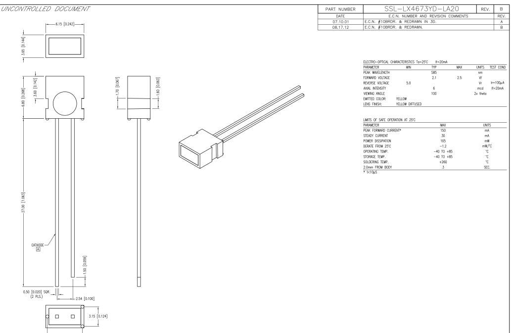
\*UNLESS OTHERWISE SPECIFIED TOLERANCES PER DECIMAL PRECISION ARE: X=±1 (±0.039), X.X=±0.5 (±0.020), X.XX=±0.25 (±0.010), X.XXX=±0.127 (±0.005). LEAD SIZE=±0.05 (±0.002), LEAD LENGTH=±0.75 (±0.030). MIN= +DECIMAL PRECISION MAX.= +0.00 -0.00 MAX.= +DECIMAL PRECISION ARE: X=±1 (±0.039), X.X=±0.5 (±0.020), X.XX=±0.25 (±0.010), X.XXX=±0.127 (±0.005). LEAD SIZE=±0.05 (±0.002), LEAD LENGTH=±0.75 (±0.030). MIN= +DECIMAL PRECISION MAX.= +0.00
