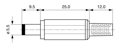
Cable diameter max. 4.0 mm
