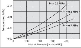
Inlet air temperature : 25°C (Saturated) Ambient temperature : 25°C Inlet air pressure
