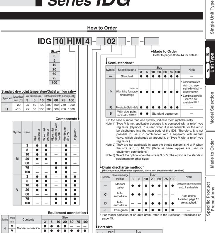
2 Μ Nipple connection Some parts of the connected contents are exceptions. Check the equipment composition (described later) or the external dimension drawing for details of the connection method and the contents of the equipmentent.
