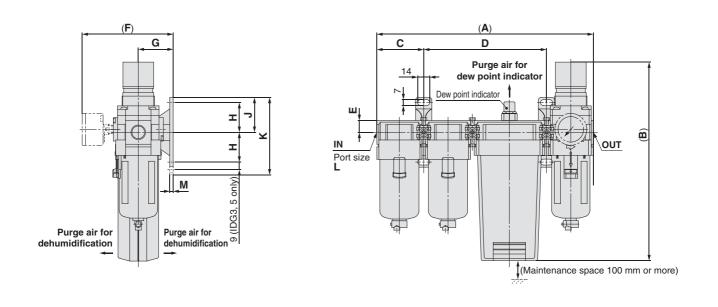
Drain Discharge (IDG3 V4, 5 V4) Drain Discharge (IDG10 V4, 20 V4) N.C.: Grey N.O.: Black Applicable tubing O.D. Rc thread or G thread: ø10 /1/8 Female thread 1/4 Female thread M5 x 0.8 NPT thread: ø3/8" Hexagon width across flats 14 Hexagon width across flats 17 Float type auto-drain N.C. type Float type auto-drain Drain guide Manual valve Drain guide Manual valve (Without drain discharge valve) (With drain discharge valve) N.O. type (Without drain discharge valve) N.C. type
