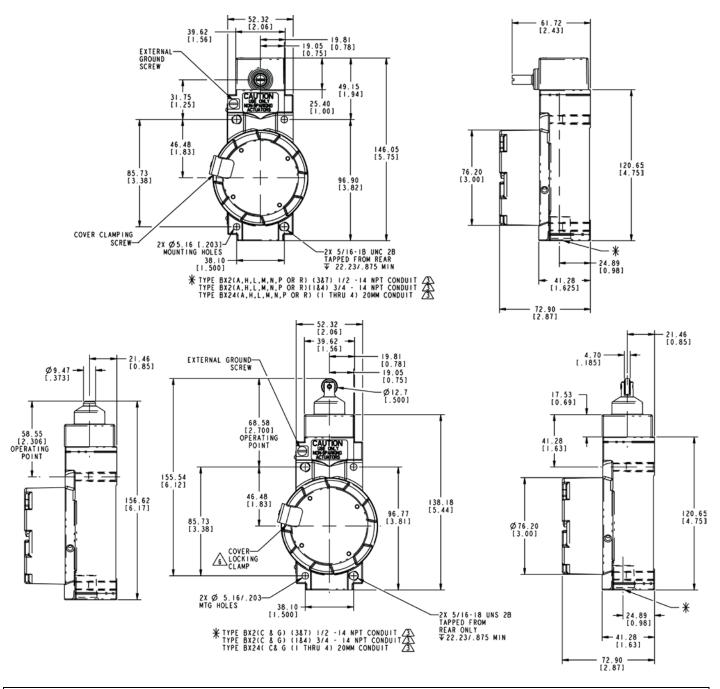
Conduit sizes 1/2-14NPT, 3/4-14NPT, M20, PG13.5, PF1/2 are available for each switch type and carry ATEX and IEC Ex approvals. 1/2-14 NPT, 3/4-14 NPT, and M20 carry UL and CSA approvals Verify that the mating threaded fitting is identical with the conduit thread shown on the product nameplate
