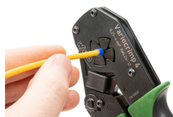
Squeeze handles until ratchet mechanism is released.
