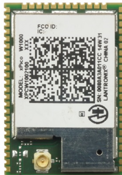
Figure 2: xPico W1003 (XPC W1003) Embedded Device Server
