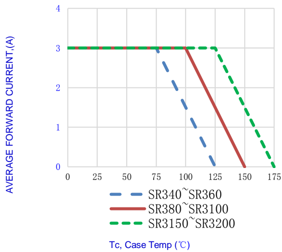
Fig.1-FORWARD CURRENT DERATING CURVE
