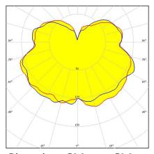
Dimensions: 56.0 mm x 56.0 mm Height: 27.30 mm ~340° omnidirectional decorative beam.
