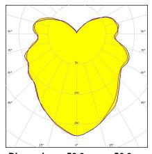
Dimensions: 56.0 mm x 56.0 mm Height: 26.70 mm ~340° omnidirectional decorative beam.
