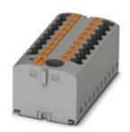
Distribution block, Basic terminal block with supply, nom. voltage: 500 V, nominal current: 24 A, connection method: Push-in connection, Push-in connection, number of connections: 13, cross section:0.14 mm² - 4 mm², AWG: 26 - 12, width: 40.6 mm, height: 21.2 mm, color: brown, mounting type: for snapping onto a DIN rail adapter, Adapter plate
