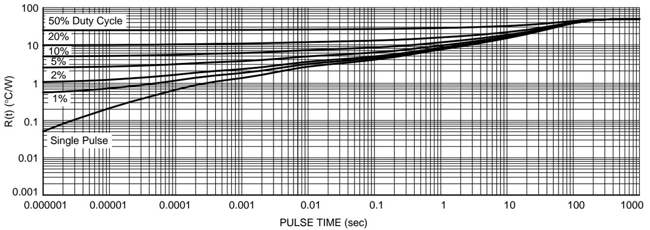
**Figure 13. Thermal Characteristics**
