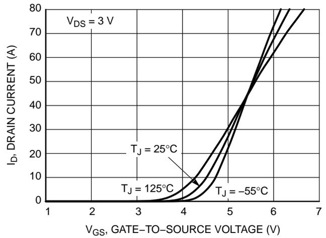
Figure 2. Transfer Characteristics
