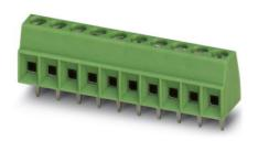
Printed circuit terminal block, nominal current: 10 A, rated voltage: 160 V, pitch: 3.5 mm, no. of positions: 5, mounting: Soldering, type of connection: Screw connection, connection direction from the conductor to the PCB:  $0^{\circ}$
