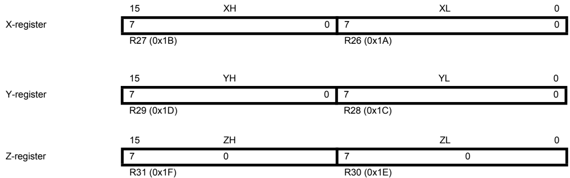
Figure 6-3. The X-, Y-, and Z-registers
