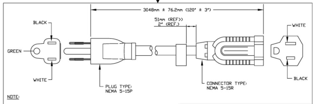
RESTRICTED USE DETACHABLE POWER SUPPLY CORD FOR BUSINESS, MAILING MACHINES AND ELECTRICAL EQUIP. THAT HAVE A BUILT IN RECEPTACLE WITH BLADES AND GROUNDING PIN FOR CORD ATTACHMENT.
