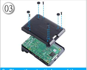
3. Place the plastic base of the NEO Case and secure the 4 screws and rubber footings.
