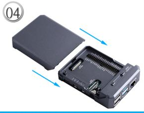
4. Slide magnetic cover to complete the NEO Case assembling.
