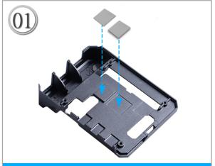
1. Align and put the thermal tapes are on the right position.
