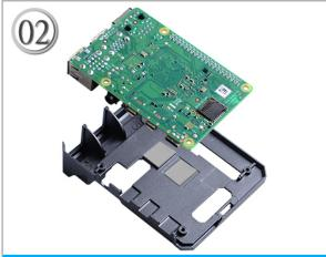
2. Align and put the Raspberry Pi on the middle of NEO Case.
