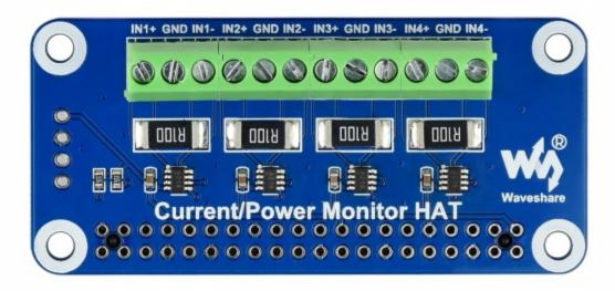
This module can be used to test currents and voltages of four channels, they are (IN1+ IN1-), (IN2+ IN2-), (IN3+ IN3-) and (IN4+ IN4-).
