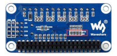
Remove the jumpers of COM-GND
