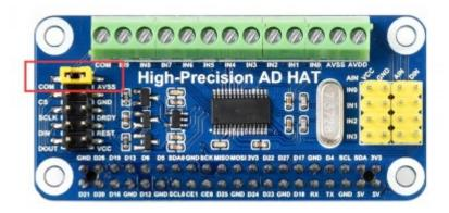
• Connect the positive end of the three-wire RTD module to IN7 and the less two to IN6 and IN4.
