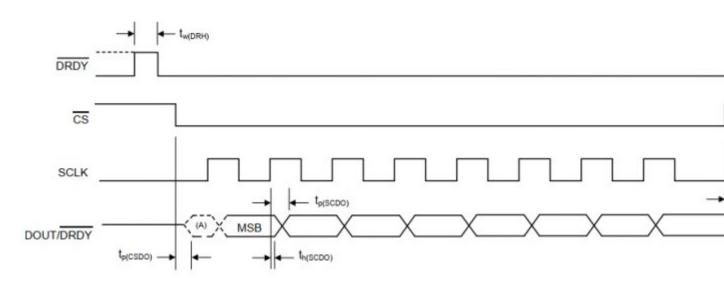
CS is chip select. The chip is active when the cs is low;
