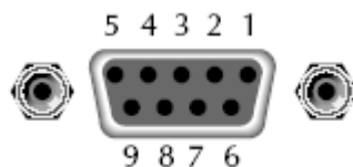
Figure 1 - RS-232 Connector Pinout
