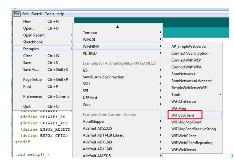
Note we use WiFiSSLClient client; instead of WiFiClient client; to require an SSL connection!
