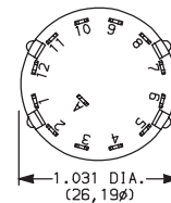
TERM. NOS. MOLDED ON HOUSING
