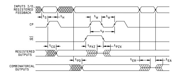
FIGURE 4. Switching waveforms.
